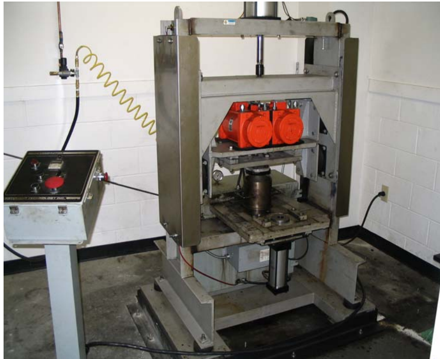
Figure 1. Vibratory Compactor used for Compaction of Test Samples
